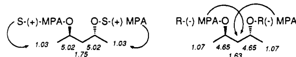
Figure 3. 1 H NMR chemical shifts of chiral Bis( O -methylmandelates) of 2( R ),4( R )-(-)-pentanediol.
